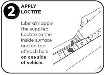
ASSEMBLE PIVOT BRACKET TO RUGGEDLINE
