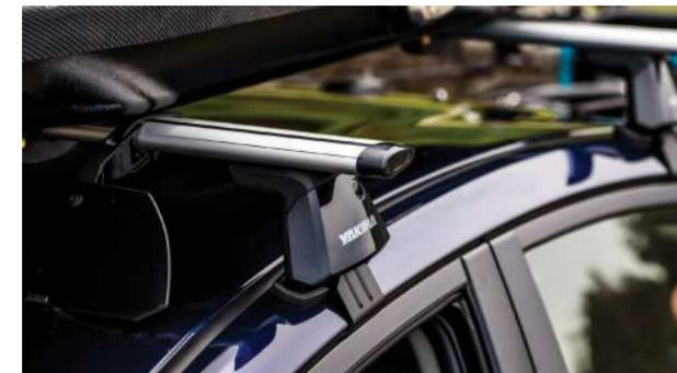
**JetStream™** - These aluminum crossbars are exceptionally aerodynamic, strong, lightweight, and really quiet. T-slot-compatible with SmartFill™ infill for efficient airflow.
